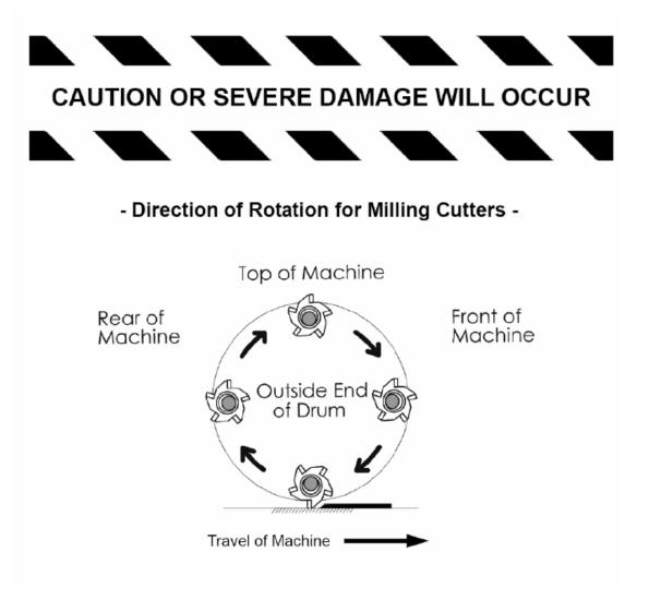
Correct rotation of the Milling Cutters is critical to successful resurfacing and to insure maximum wear life. Drum and cutter assembly should be mounted so that cutters are rotating towards the front of the machine as indicated above.
