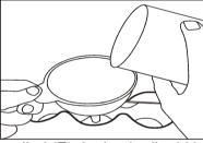
4.3 Using the lighter supplied (E), ignite the liquid in the reservoir by bringing the flame close to the surface of the liquid.
