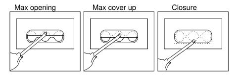
Closing the reservoir shutter completely will cause the flame to be extinguished.
