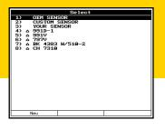
The ACES Systems Model 2020HR allows you to define a list of your sensors, which is then stored so you can change sensor types between jobs. The Model 2020HR stores all the information you need to balance, track, or perform vibration surveys on your entire fleet.
