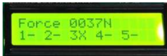
Figure 4.2 – Bottom LCD screen on main console during ‘Train Like a Pro’ mode.
