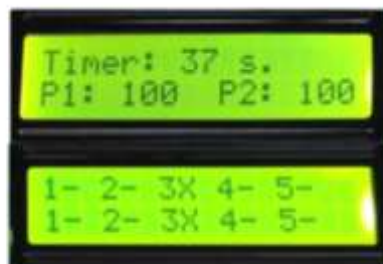
Figure 4.1 – Top and bottom LCD screens on main console during Multiplayer Combat mode.
