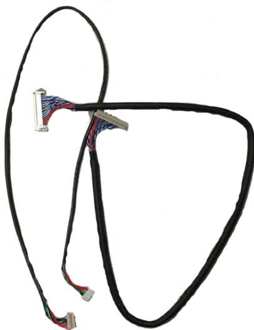
Figure 11: LVDS Cable and LVDS Backlight Cable
