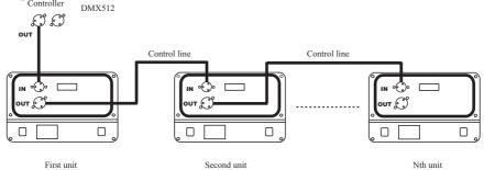
Caution: Please remember the signal output of last machine must connect the attached circle plug .The circle plug connect a 120 resistor between 2 feet and 3 feet canon plug. The signal reflects phenomena can be avoided by using circle plug during DMX 512 signal transfer.
