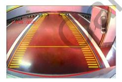
In V-POSITION use  $\triangle$ ,  $\bigtriangledown$  on remote control, to adjust parking guideline up and down.
