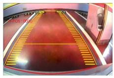
In H-POSITION, use  $\triangleleft$ ,  $\triangleright$  on remote control, to adjust parking guideline left and right.
