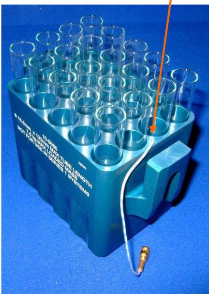
**SampleGuard** is a dual channel temperature monitoring system that operates when the rotor spins. One channel allows the evaporator to control the temperature of a sample holder, the other monitors the temperature of a sample within the holder.
