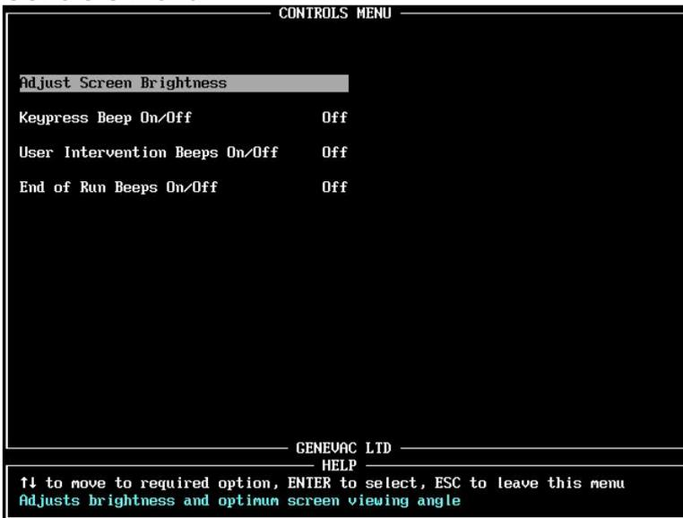
**Adjust Screen Brightness:** Adjusts the screen viewing angle. The function is not available on newer instruments fitted with high contrast screens.
