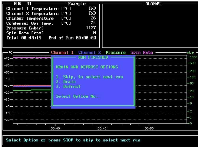
Select **Skip**, **Drain** or **Defrost** using the numeric keys indicated.
