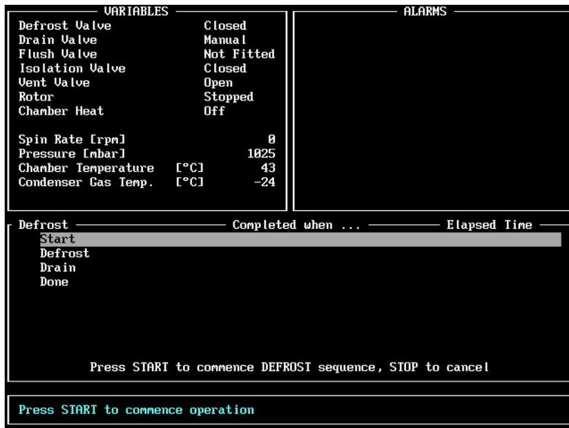
The evaporator defrosts the condenser until solvent defrost is automatically detected. Alternatively, press the **STOP** key to end the defrost cycle.
