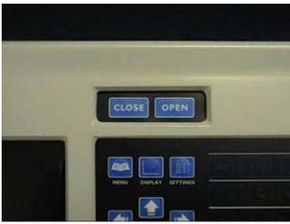
Press the **Open** key on the front panel to unlock the door and open the door manually.
