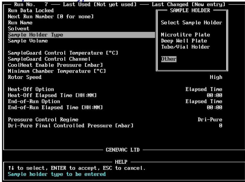
Select a sample holder type from the window that opens. If the required sample holder option is not available, select *other* and enter the details (no more than 31 characters).
