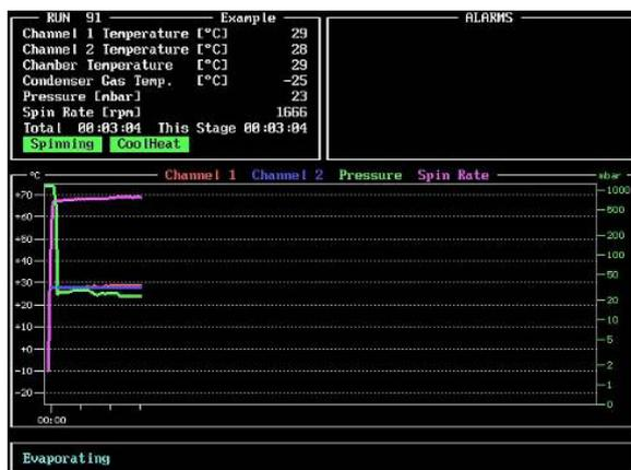
The **Run Log** screen is displayed whilst a run is in progress. It shows the current status of the evaporator in numerical and graphical form. When the SampleGuard probes are appropriately configured, it is possible to extrapolate information from the graph that relates to sample drying progress. An evaporative cooling effect can be seen in the divergence of the channel 1 and channel 2 traces. Conversely, converging traces reveal when a sample is dry. See **Using SampleGuard** for details.
