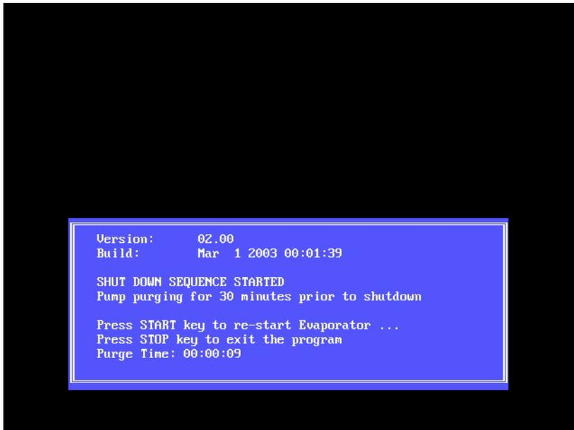
The evaporator continues to purge the vacuum pump for a time period indicated on the screen. Press the **START** key at any time to restart the evaporator.
