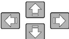
Press the **cursor direction** left and right keys to highlight the options on the horizontal menu bar near the bottom of the screen. Press the up and down keys move the **white band** cursor.
