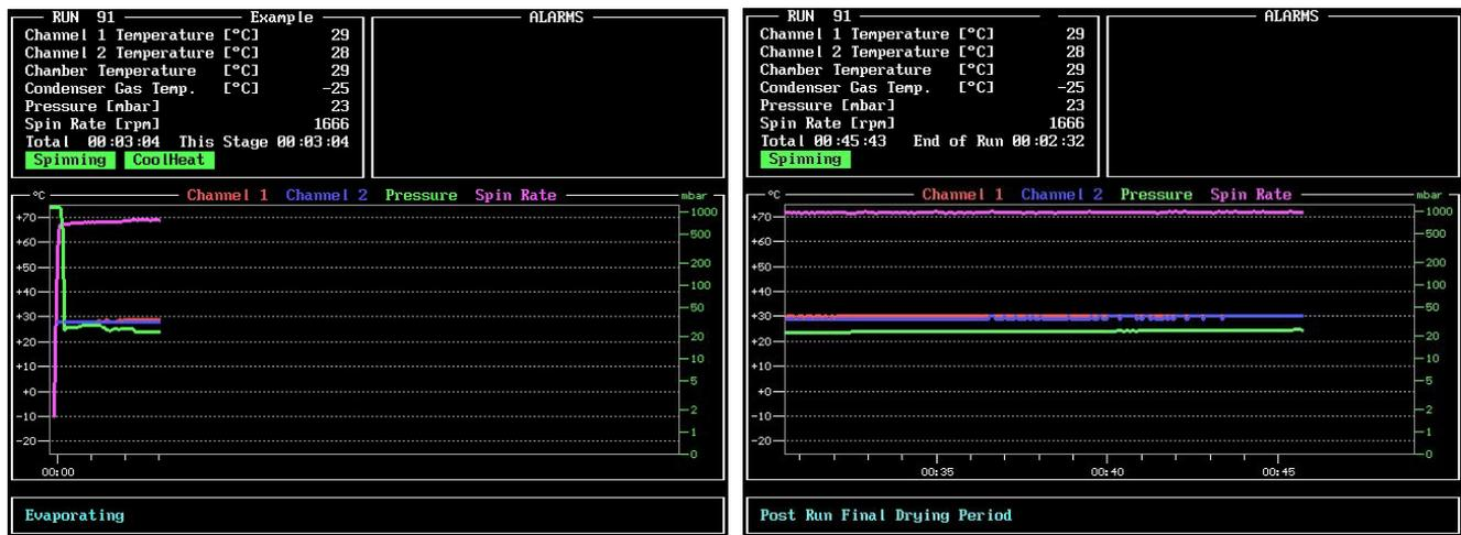
Press the **DISPLAY** key during a run to return to the **RUN LOG** screen.
