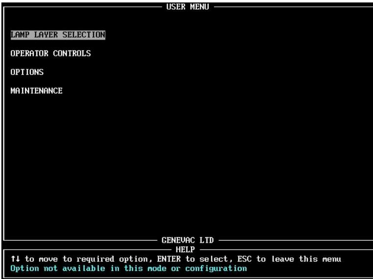
**Lamp Layer Selection:** Disable associated lamp layers if 2<sup>nd</sup> or 3<sup>rd</sup> rotor levels are not used.
