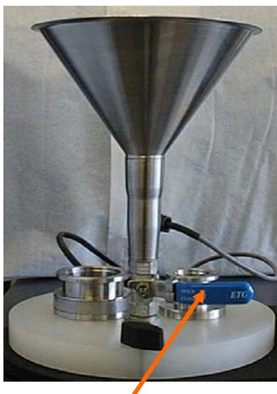
Use the condenser flusher (if fitted) to clean traces of volatile solvent from the condenser before evaporating a less volatile solvents, the condenser operates most efficiently when it is drained and clean.
