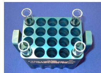
Rotate the rotor by hand. Check that all tube holders and plates are correctly located and swing freely. Use only the sample holders supplied with the system, or that are specified for use with the system. Never use non Genevac approved sample holders.
