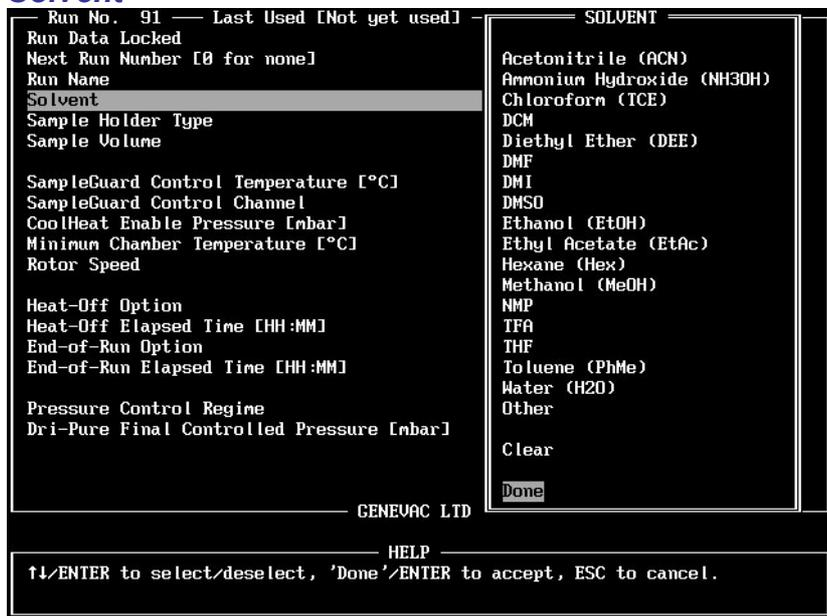
Select a solvent from the window that opens. More than one solvent may be selected if using a mixture of solvents. Selected solvents are highlighted in blue. Select **Done** when the solvent or solvents have been selected. Alternatively, select **Other** and enter the solvent name (no more than 31 characters).
