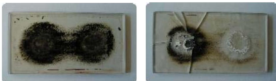
Whilst the solvent evaporates, the product becomes carbonised by the heat from the lamps and forms sites where crack propagation can occur. Inspect the lamp glass at regular intervals and clean with a lint free cloth and acetone.
