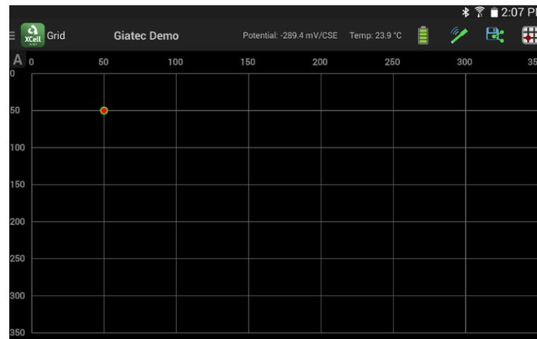
**⚠** The user can re-test any previously tested location. To do so, simply move the probe to the location you want to re-test.
