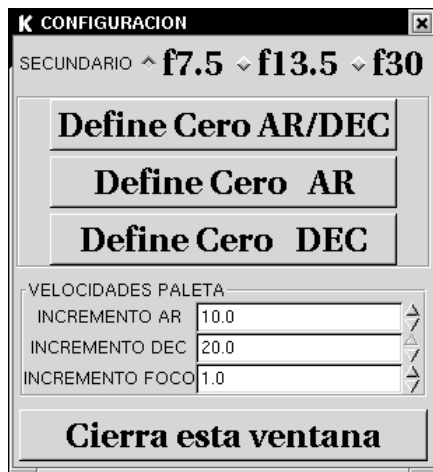
Figure 5. Configuration window in the GUIADOR 2M (Motores) window. The use of the VELOCIDADES PALETA is of particular importance in spectroscopical observations.
