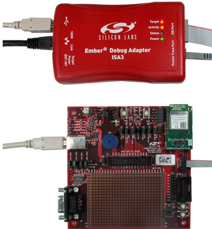
Figure 15. Debug Adapter (ISA3) Supplying Power; FTDI Serial <-> USB Converter Used for Communication
