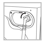
2. Connect the other end of the water inlet hose to the washing machine, screwing it onto the applian-
