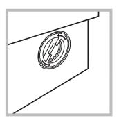
2. unscrew the lid by rotating it anti-clockwise (see *figure*): a little water may trickle out. This is perfectly normal;
