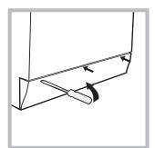
1. using a screwdriver, remove the cover panel on the lower front part of the washing machine (see figure);
