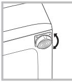
1. Install the washing machine on a flat sturdy floor, without resting it up against walls, furniture cabinets or other. 2. If the floor is not perfectly level, compensate for any unevenness by tightening or loosening the adjustable front feet *(see figure);* the angle of inclination, measured according to the worktop, must not exceed 2°.
