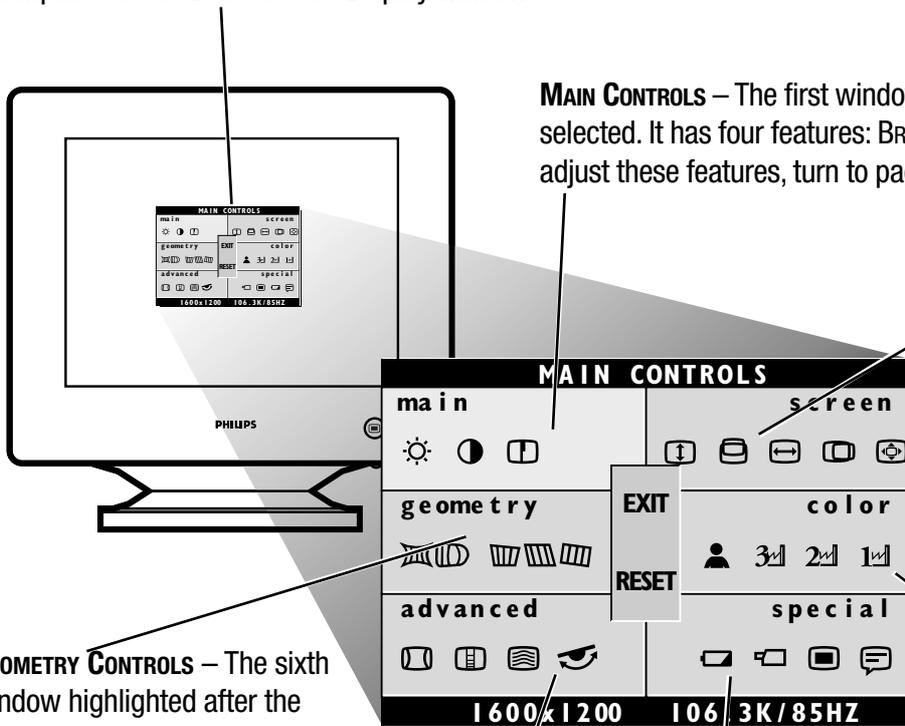
**MAIN CONTROLS** – The first window highlighted after the OSD has been selected. It has four features: BRIGHTNESS, CONTRAST and DEGAUSS. To adjust these features, turn to pages 4 - 5.
