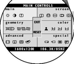
**2** Turn the ROTARY knob until the COLOR TEMPERATURE window is highlighted. Then press the On SCREEN DISPLAY button.
