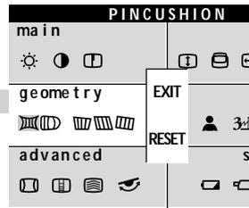
**2b** Press the On SCREEN DISPLAY button. Then, turn the ROTARY knob to adjust the pincushion.
