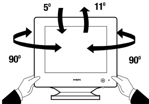
**PEDESTAL** – With the built-in pedestal, you can tilt and swivel the monitor to the most comfortable viewing angle. To best use your monitor, always place it at eye level.
