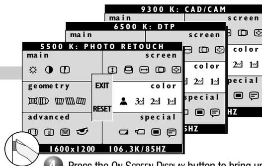
**4** Press the On SCREEN DISPLAY button to bring up and save the preset settings for 9300 K CAD/CAM, 6500 K DTP, or 5500 K PHOTO RETOUCH.
