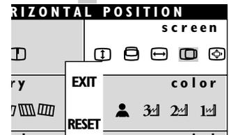
**3** Press the ON SCREEN DISPLAY button to bring up HORIZONTAL POSITION screen.
