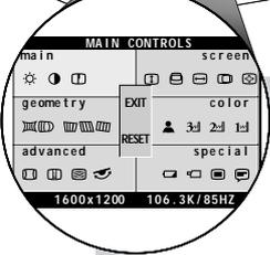
**2a** Turn the ROTARY knob until the GEOMETRY CONTROLS window is highlighted. Next, press the On SCREEN DISPLAY button. Then, if necessary, turn the ROTARY knob until PINCUSHION icon is highlighted.
