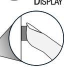
**2** Turn the ROTARY knob until the SCREEN SIZE & POSITION window is highlighted. Next, press the ON SCREEN DISPLAY button. The FULL SIZE icon is highlighted.
