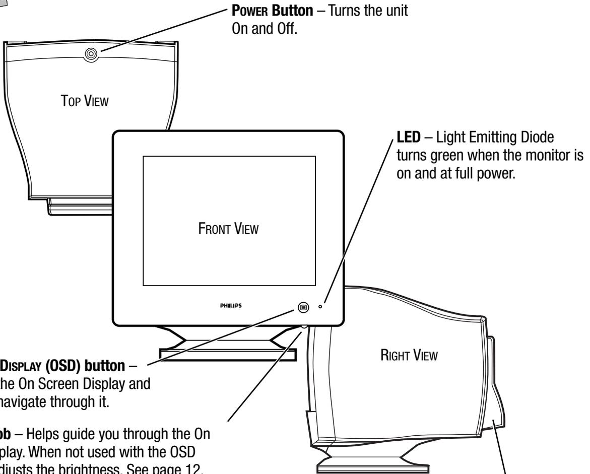
**CABLE COVER** – Snaps onto the back of the monitor to conceal cable connections. (Cable connections shown in the manual are without the cover on.)
