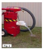
When ground water or other sources of water infiltrate the excavation, the dewatering attachment allows the hopper to collect both solids and water. Water is naturally decanted and released out of the hopper each time the system is idled (each time the control valve is released). Outlet is standard 6" Schd 40 female slip fitting which must be equipped with a check valve for water pumping operation. The discharge is gravity flow.
