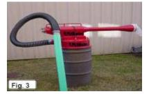
Typical Applications: Drums are used when material needs to be hauled off site, or when material will be packed into drums for disposal. Although the top of the VE-75 hopper fits the top of 55 gallon open top shipping drums the VE-55 system provides better separation and allows drums to be filled to the top.
