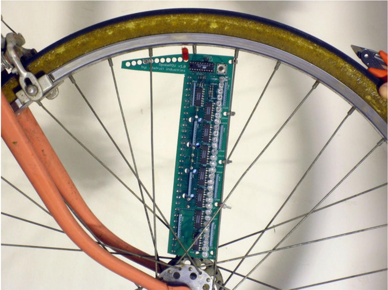
Attach the magnet to your frame. If you have a steel bike, this is really easy. You want to make sure that the south side of the magnet is facing out since the sensor is sensitive to the south side only. Try to put the magnet as close to the sensor as possible. Press the button to turn on the SpokePOV and try moving the wheel back and forth around the magnet, you should see the LEDs start to blink.
