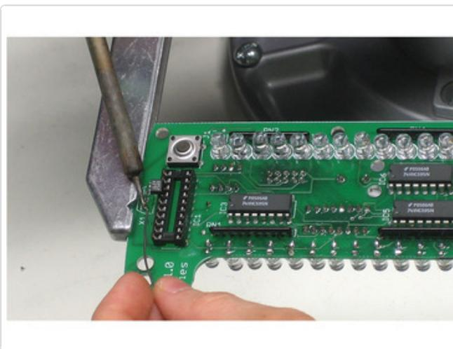
Bend the sensor so that the face points out as shown. Since the sensor has to stick out but has short leads, solder it from the top, making sure that the leads don't stick too far through on the other side. See the picture to the left.
