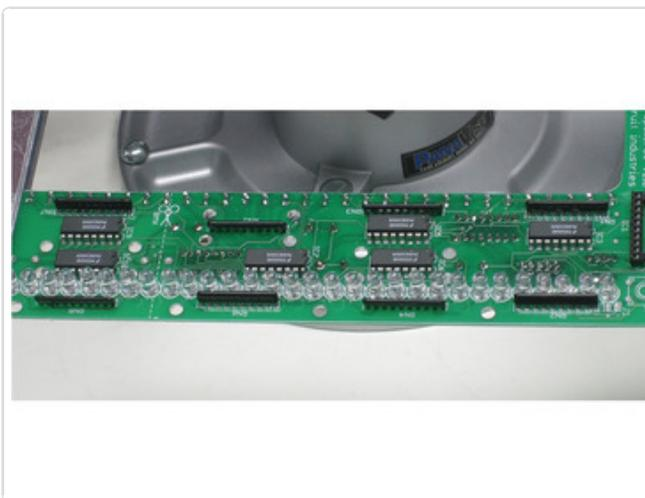
Solder in the 8 9-SIP resistor networks. Make sure you align them correctly: one side of the resistor pack has a dot which corresponds to pin 1 which is marked with an X in the picture on the circuit board.
