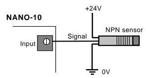
Input = logic '1' when Limit Switch is closed
