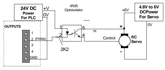
Figure 11.5 Opto-Isolated Interace to RC Servo
