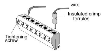
Figure 1.3 – Using Ferrules to connect to screw terminal block
