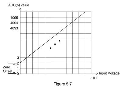
The zero offset error can be corrected by entering a value into the "ADC Zero Offset" field. Any number between -100 and 100 can be entered here. The ADC(n) function would add the zero-offset value that you entered here to the measured value and return the total sum to the calling routine.
