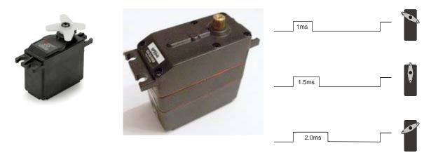
Figure 11.3 RC Servo and Control Signal
