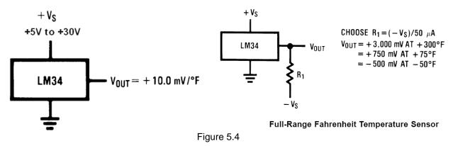
The LM34 is a wonderful, low cost semiconductor temperature sensor with a range of -50 °F to 300 °F. It is extremely easy to use for measuring temperature above 0 °F. You simply connect one pin to the
