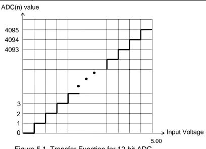
Figure 5.1 Transfer Function for 12-bit ADC.
