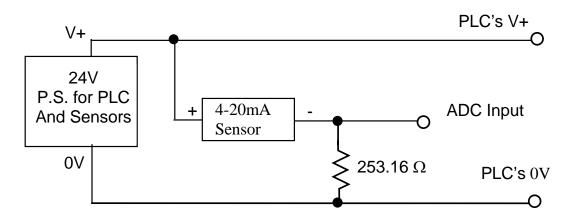
\* Use a 250.0 + 3.16 ohm resistors in series to obtain 253.16 ohm.
