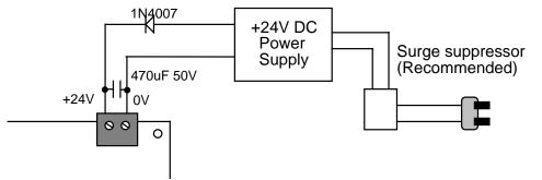
To ensure that the power supply provides a slow voltage gradient during power down, the power switch must be connected to the AC side of the power supply instead of to the DC side of the power supply. All industrial DC power supplies usually have large filtering capacitors at the DC output, which means that the power supply to the load would normally decrease slowly when power supply to the AC side has been cut.
