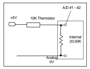
Figure 5.6: Connecting 10K Thermistor to NANO-10 ADC# 1-2
