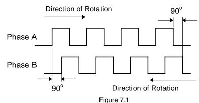
When the encoder shaft rotates in one direction, phase A leads phase B by 90 degrees. When the shaft rotates in the opposite direction, phase B will lead phase A by 90 degrees. The quadrature signals therefore provide an indication of the direction of rotation.
