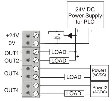
Figure 1.6 – Nano-10 Output Interfacing to Load
