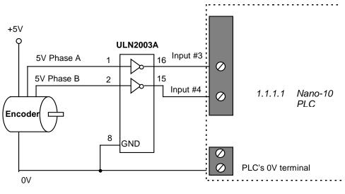
Figure 7.2 Interfacing 5V type Rotary Encoder
