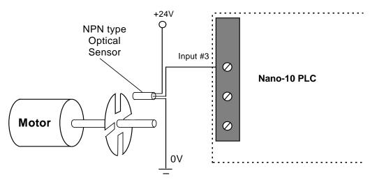
Figure 8.1 Setting Up a Simple Tachometer or Encoder
