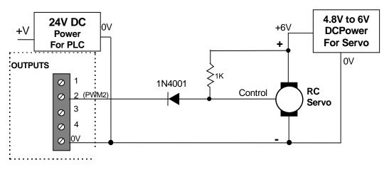
Figure 11.4 Non-isolated Interace to RC Servo
