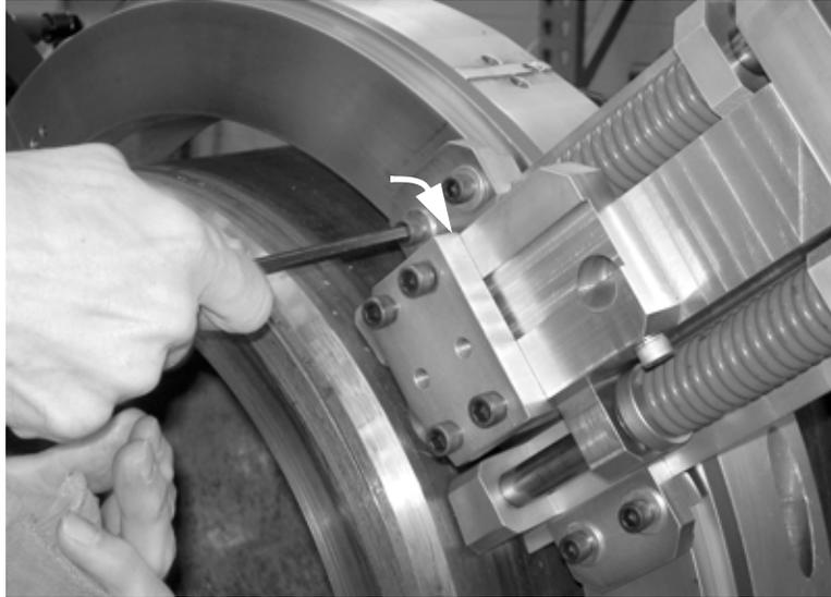
*Figure 3-12. Once the slide positions are set, securely tighten the mounting clamp screws.*
