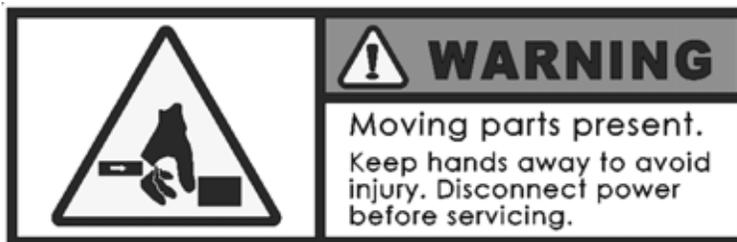
*Figure 2-2. The Moving Parts warning label is on the trip assembly (part no. 03-113-04).*
