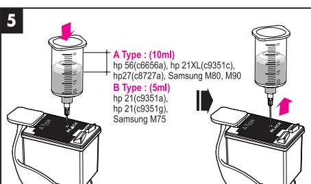
**5** Pull up the injection needle about 5mm backward, and inject the recommended ink volume according to your cartridge model number by pressing the piston of the ink container for about 20 seconds. Then pull out the ink container.
