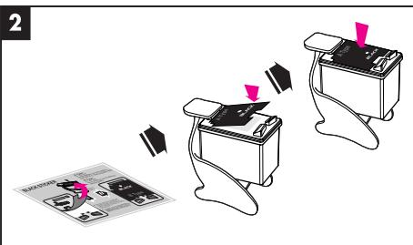
**2** Please check the correct type of the supplied injection inlet sticker according to your cartridge model number. Attach the correct type of the injection inlet sticker on the label of the cartridge cover in the right direction as shown in the figure.
