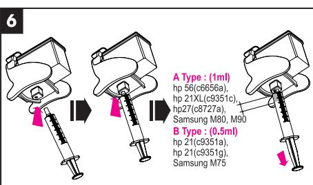
**6** Connect the supplied suction syringe to the rubber hole on the bottom of the refill clip, and slowly suck out the recommended ink volume according to your cartridge model number. Then remove the syringe.
