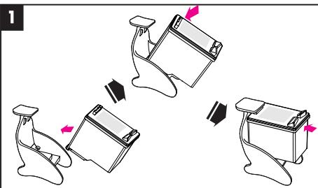
**1** Insert the nozzle part of the cartridge into the refill clip, and push the top of the cartridge all the way in until you hear it clicking into place.
