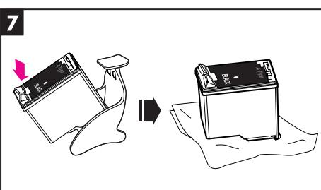
**7** Remove the cartridge from the refill clip and clean the excessive ink around the nozzle, dabbing the nozzle part of the cartridge on some sheets of soft tissue. Install it in the printer, and then run the "cartridge cleaning" process before use.
