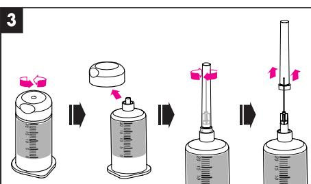
**3** Open the cap of the ink container and connect the ink injection needle.
