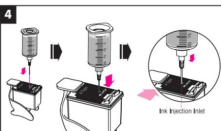
**4** Insert the injection needle deep into the ink injection inlet marked on the sticker with the needle directed toward the nozzle.
