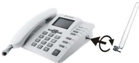
Position the antenna upwards at its connecting joint. This will ensure optimal reception.
