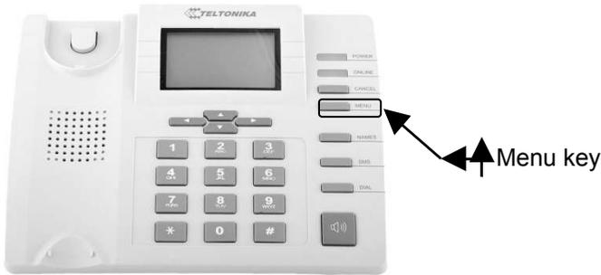
Menu items are selected by using up and down arrow keys ▲ ▼ located below the LCD screen.
