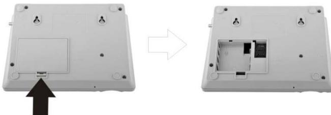
3. Flip SIM card holder and gently insert SIM card in the slot
