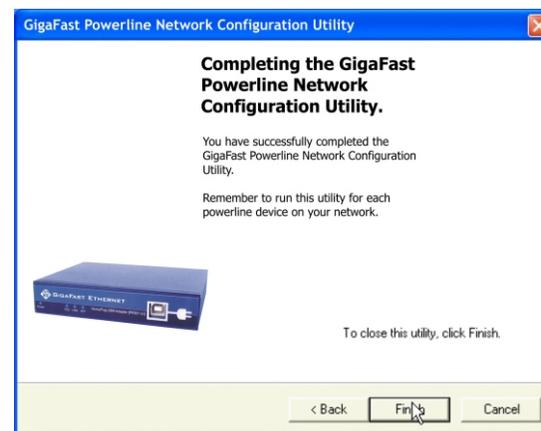
Upon completion of the installation, this program does not need to be run again unless the encryption is to be changed. The HomePlug adapter will not lose its encryption key by unplugging the power, so the unit can be setup and moved to the correct location.
