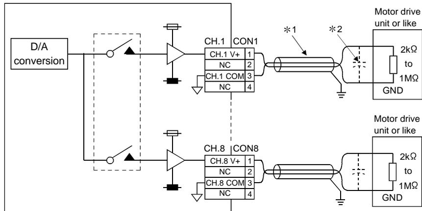
\*1 Use a two-core twist shielded line for the wiring.
