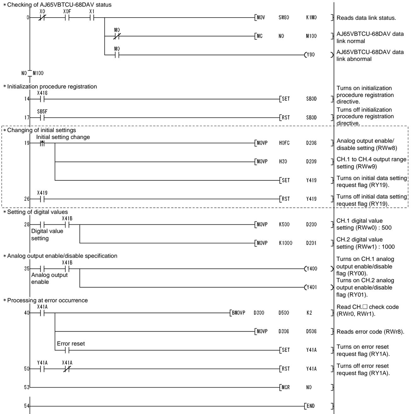
\* The program enclosed by the dotted line is necessary only when the initial settings are changed.
