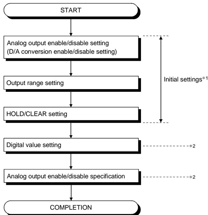
\*1 When using the QCPU (Q mode), you can use the remote device station initialization procedure registration function to make settings. When using the ACPU, QCPU (A mode) or QnACPU, use the sequence program to make settings.
