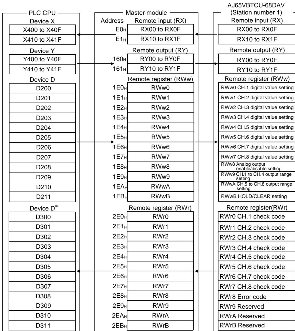
\* In the program example (refer to Section 5.5) that uses the RRPA instruction (automatic refresh parameter setting) with the ACPU/QCPU (A mode), RWr0 to RWr8 are assigned to D456 to D464.
