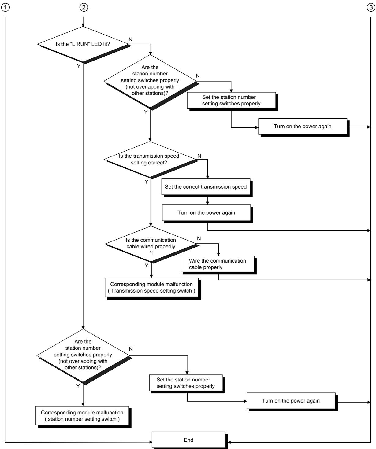
\*1Check for a short, reversed connection, wire breakage, terminal resistor, FG connection, overall distance and station-to-station distance.
