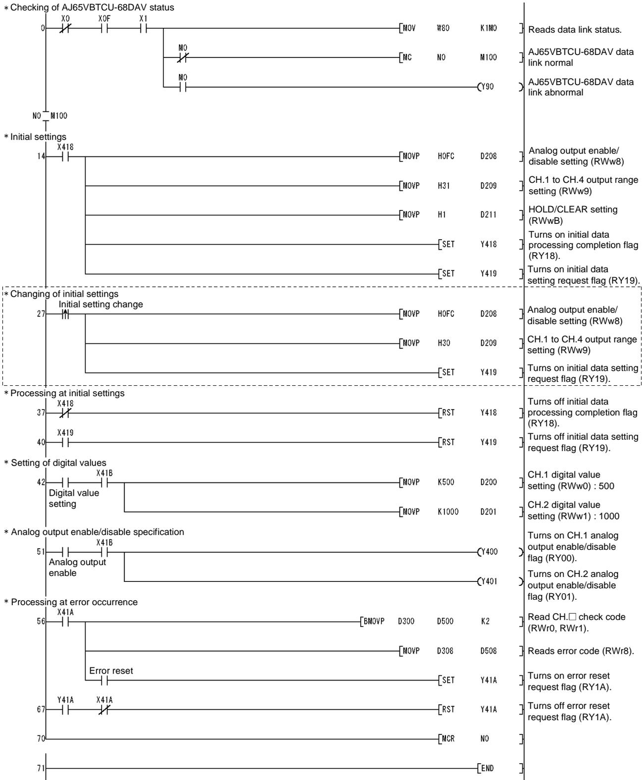
\* The program enclosed by the dotted line is necessary only when the initial settings are changed.
