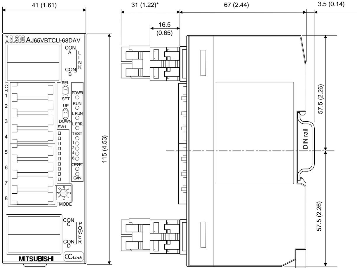
\* :This section should be 14.5mm (0.57inch) when an online connector is not installed.
