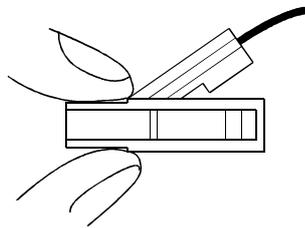
Insert the signal cables into the one-touch connector plug as shown below.
