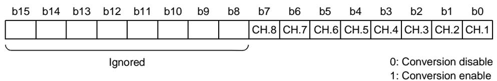
3.6.4 CH.  output range setting (Address RWwm+9, RWwm+A)
