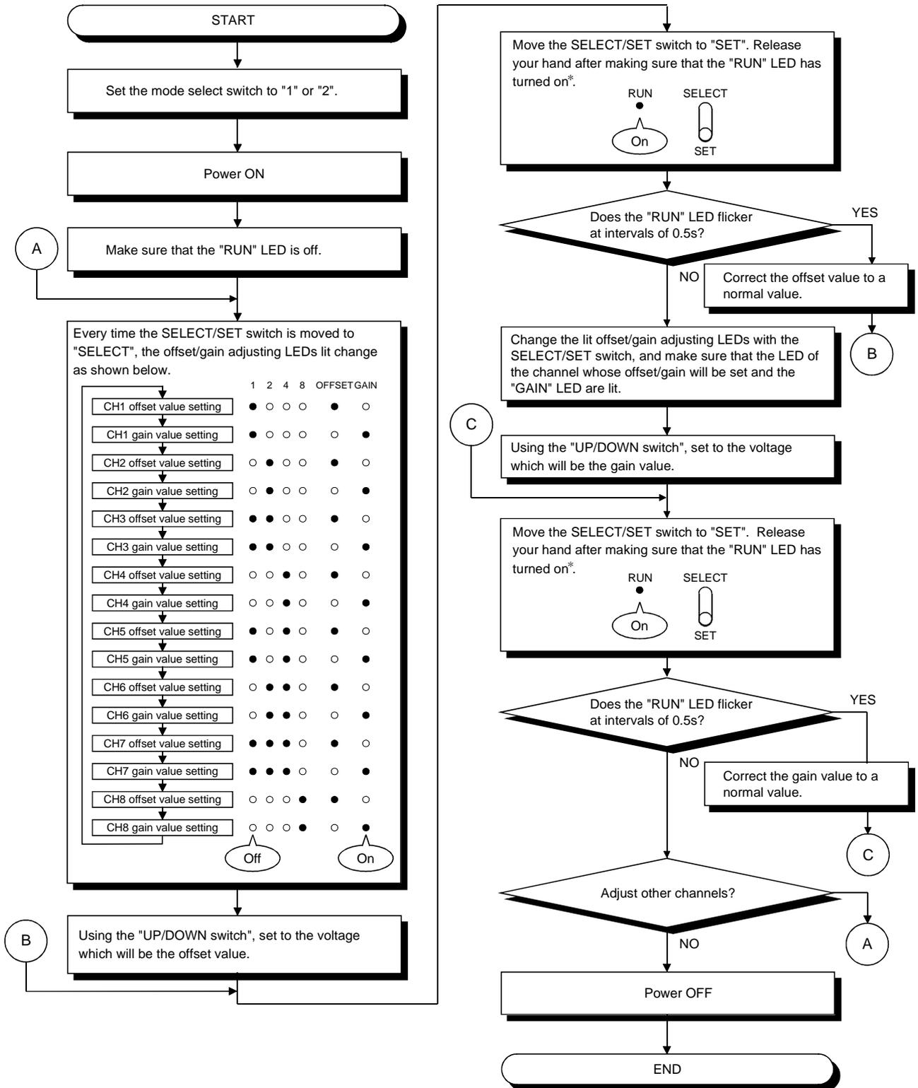
\* If the "RUN" LED is not lit, E<sup>2</sup>PRON may have failed. For details, refer to Section 3.5.2.
