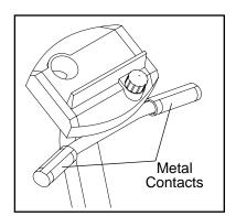
inner contacts and your fingers must be touching the outer contacts. Avoid moving your hands. After a moment, the heart indicator in the PULSE display will flash and your heart rate will be shown. For the most accurate heart rate reading, continue to hold the contacts for about 15 seconds.
