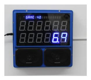
The system CPU contains the main electronic boards, the sound system and speakers, the time clock, the scoreboard, the touch key interface for making game and systems selections, the power supply and the recharging unit for the wireless play pods.
