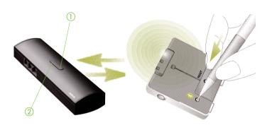
Initiate the pairing process on your iCom by pressing the Bluetooth pairing button for about 2 seconds until the Bluetooth indicator flashes blue. Your iCom will remain in pairing mode for two minutes or until the pairing is completed.
