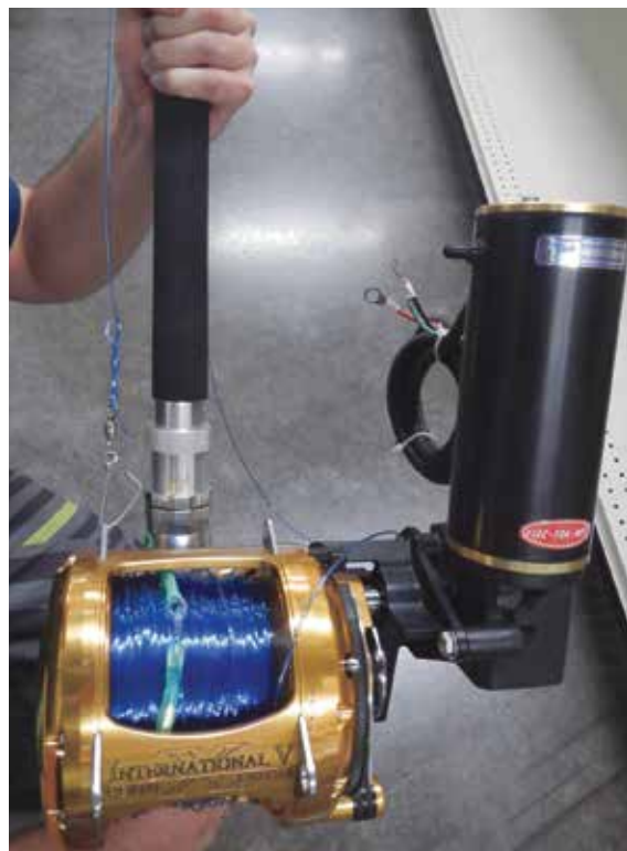
Light Style: 130 lb class greenstick rod and Penn International (130) with Electramate 1380GH motor.
