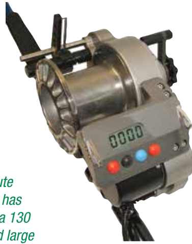
The Lindgren-Pitman S-1200 electric reel (12VDC motor). Note: a modified level winder may be needed for knot clearance.
