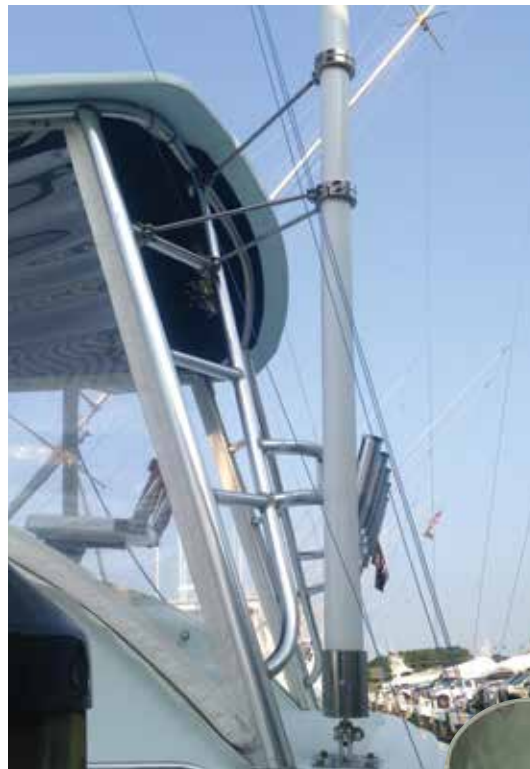
Two examples of custom built (DIY) upper support clamps, when a U-Bolt just won't do.
