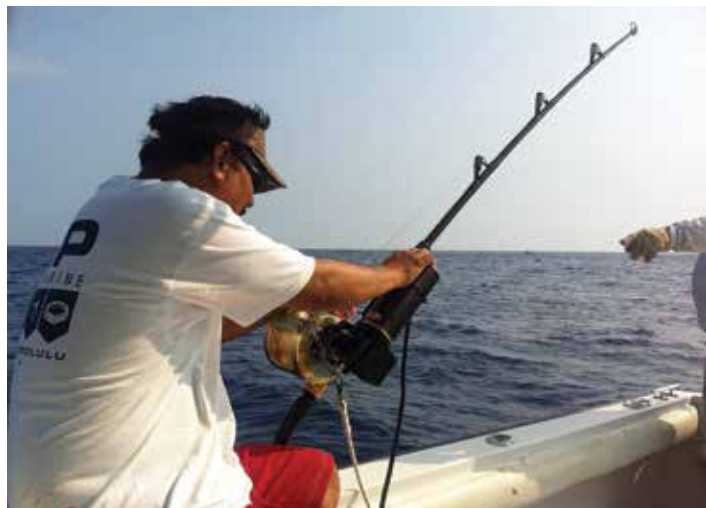
Shimano Tiagra (130) fitted with an Electramate 1380GH motor and a modified 130 lb class trolling rod, with extra wide roller guides and tip.
