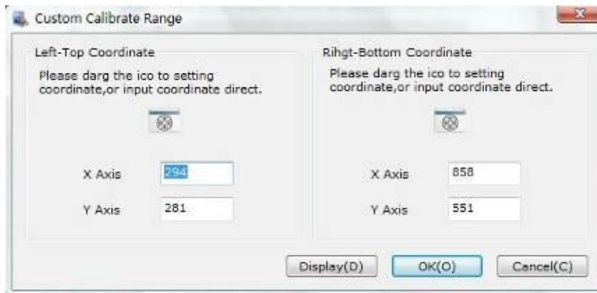
4 points calibration: calibrate by 4 points, for 4 WIRE RESISTIVE and Infrared touchscreens.
