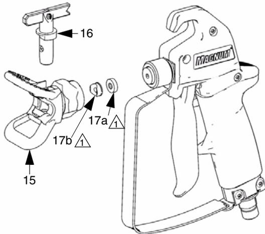
1 Always replace the gasket and seat (included with tip) when you replace a worn spray tip. See **Installing Tip (16) and Guard (15) on Gun**, page 2.
