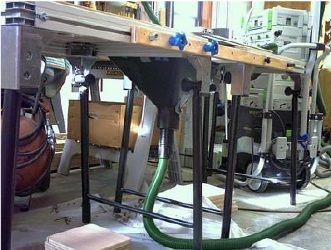
Bottom mounted Dust Collection
