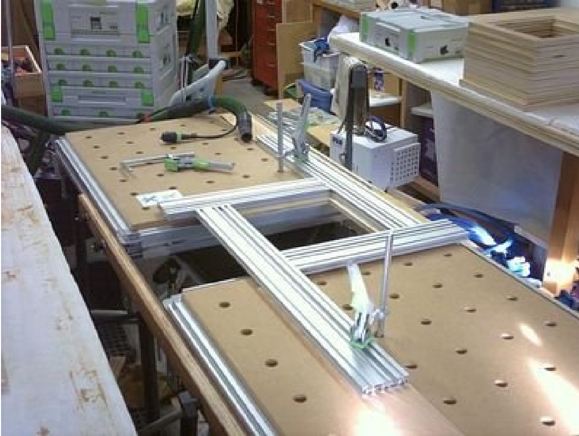
Pair of Joined MFT 800s, view from topside.
