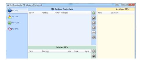
(This is what a blank FlashScan V2/AutoCal would look like, it's ok to have PID groups already in there for other controllers, however for maximum scan rates existing 6.7L CMD PID groups should be removed).
