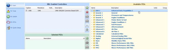
NOTE: Individual PID's cannot be added / removed from the EDA scan group, trying to do so will not improve logging speeds.
