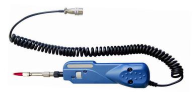
FIM-2 video microscope is used to inspect end-face of fibers and check the optic connectivity. It magnifies fibers of 125um diameter 650 times, enlarging picture through a video signal to the display where the status of fiber end-face is showed clearly in the end.
