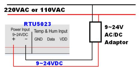
• If you want to use the RTU5023 to monitoring 9~24VDC power status or voltage, please connect the DC power to RTU5023 directly, for example, solar panel or battery or equipment status. And setup it is threshold value by SMS commands. See below. Connection:
