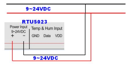
In this condition, the RTU5023 was powered on by the 9~24VDC directly
