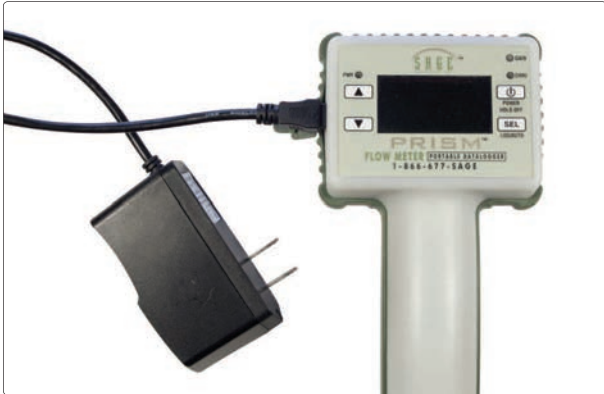
Meter Shown with PowerPak for Charging
