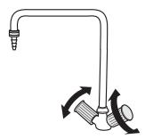
Open/close mixer water taps with levers and temperature adjustment
