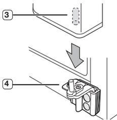
3. Insert the upper hinge shaft **5** into the hole on the hinge **6**. Make sure the hinge is level between the upper hinge hole **7** and the hole on the top of the cabinet **8**. Then, reattach hinge screws **9** and the ground screw **10** by turning it in a clock wise direction.
