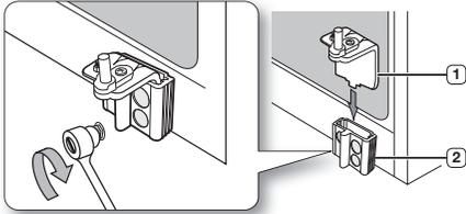
2. Fit the hole in the corner of the fridge door **3** over the lower hinge **4**.
