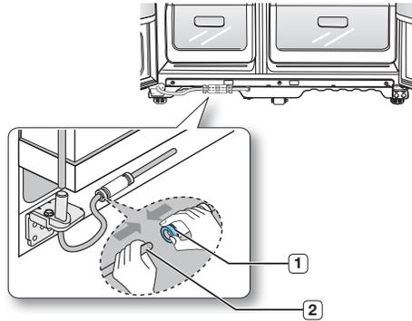
2. The Water Line must be fully inserted to the center of transparent coupler to prevent water leakage from the dispenser.
