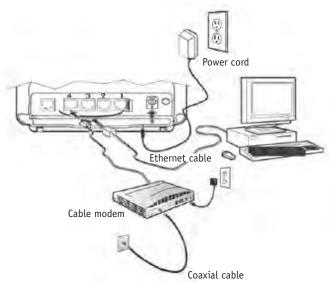
**Important note:** The Cable modem must be connected in the #4 port of your wireless modem router.
