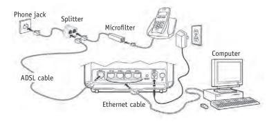
**Important note:** If you are plugging in or adding phones, it is important to have a Microfilter which support ADSL technology on each phone.
