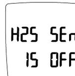
To enable H<sub>2</sub>S sensor repeat above sequence. The display advises H<sub>2</sub>S Sensor is ON.
