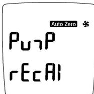
Then, the audible alarm beeps twice, the pump icon stays lit, the auto span icon flashes and the display shows:
