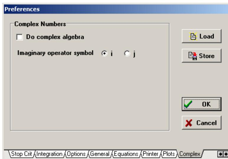
The **Complex Numbers** Tab allows the complex algebra capability in EES to be turned on or off. The complex capability can also be turned on or off with the \$COMPLEX ON/OFF directive. The imaginary variable name representing the square root of  $-1$  can be designated to be either  $i$  or  $j$  depending on the radio button setting. Complex mode can also be turned on or off but clicking on the Complex field in the status bar of the Equations window.
