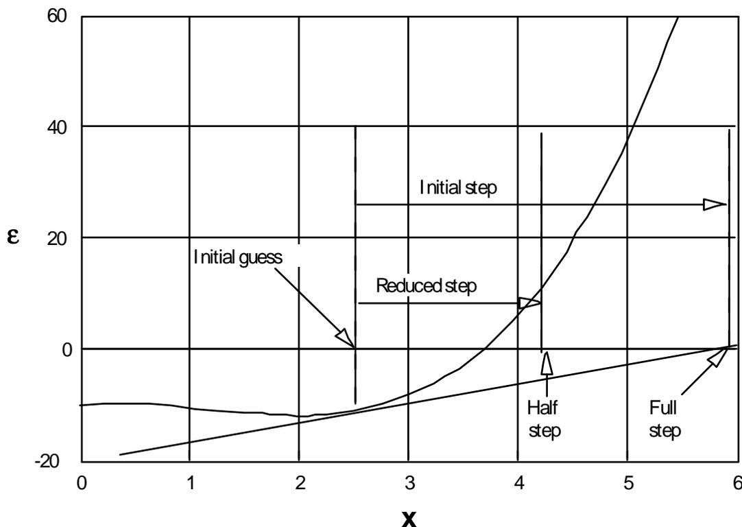
Figure 2: Use step-halving for improving the convergence
