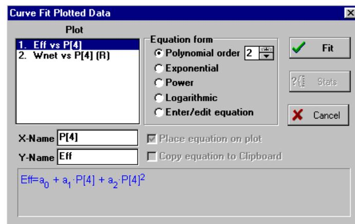
Click the Fit button (or press the Enter key). The fitted equation will be displayed in the box at the bottom of the dialog window. A Stats button will appear. Clicking the Stats button will display the following statistical information relating to the curve fit.
