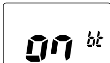
Battery voltage indication ON
