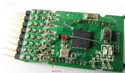
Figure 4-8 Installing a Diode for RSSI Measurement
