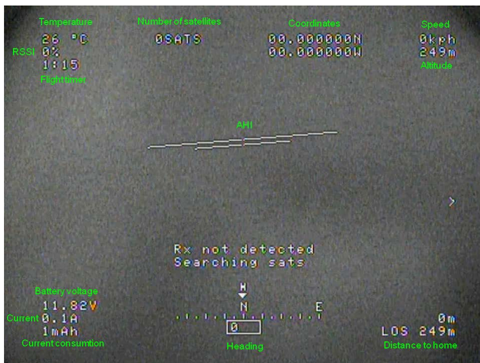
Figure 3-18 On Screen Display Description (Simple)
