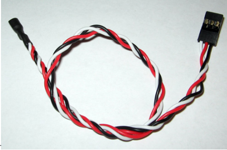
Figure 3-5 External Temperature Sensor
