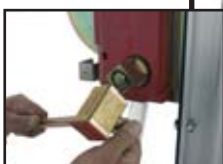
High capacity winch with dismantled crank.
