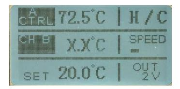
Temperature is not only controlled for A but can be controlled for B as well when B is put in control mode. Once in control mode, you can change the temperature for B by using the arrows when no option is highlighted.
