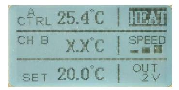
Using the arrows above and below mode, the heating and cooling function can be changed to the desired function.
