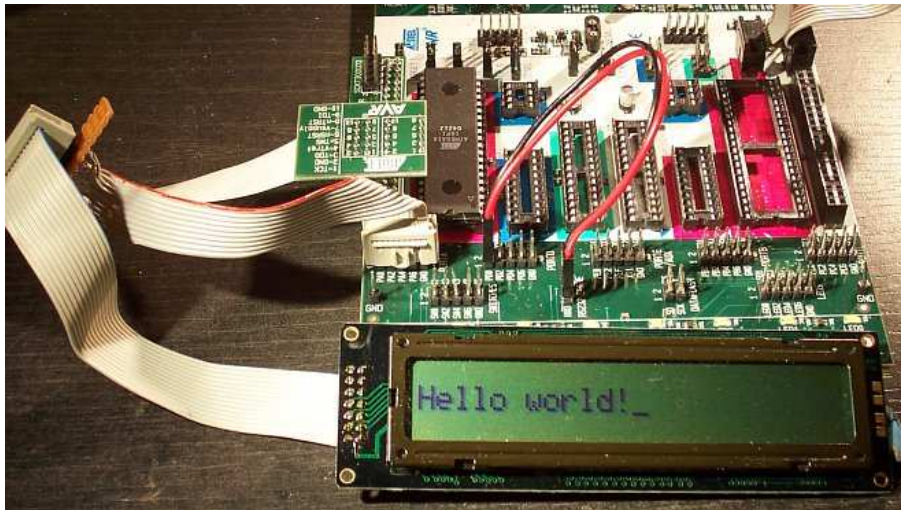
Figure 9: Wiring of the STK500
