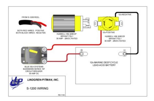
Power Requirement and Wiring: 12-volts DC Max 30Amps Plug – Hubbell #HBL328DCP Available Receptacle – Hubbell #328DCR
