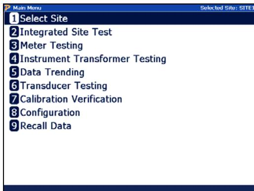
25. Select the site that was tested and review the data before leaving the site. Use up and down arrows to select the site and F6 to expand and view the data. After review is complete, power off the PowerMaster<sup>®</sup> by pressing the ON key.
