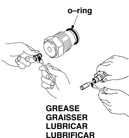
6. Grease o-rings on diffuser and new needle using a *nonsilicon* grease.
