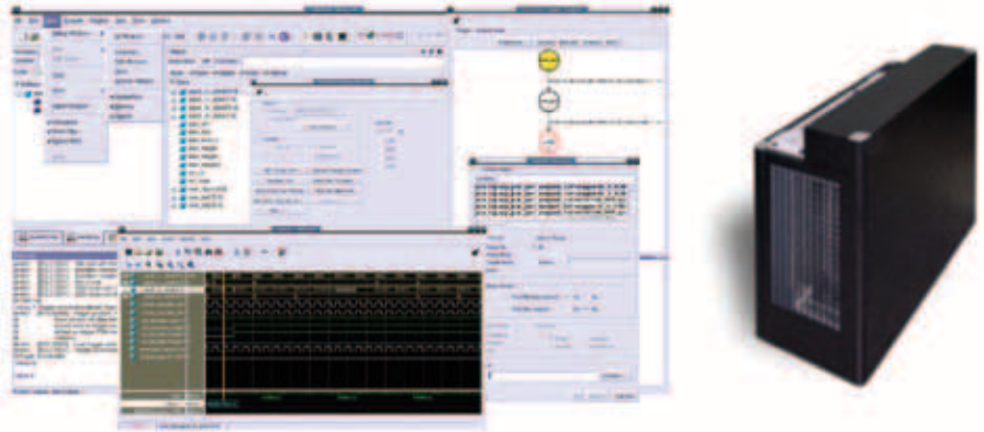
Figure 2: Veloce hardware emulator and its debug application environment
