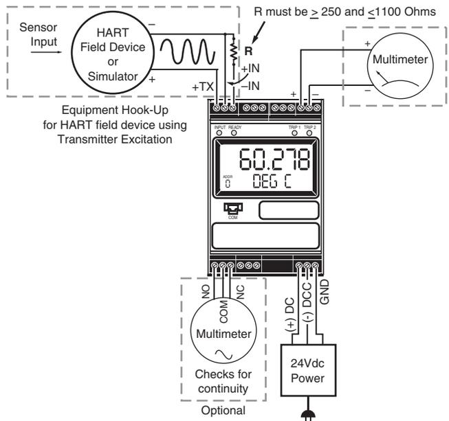
Figure 5. Installing a HIM Into the Loop Using an External Power Source to Power a Transmitter
