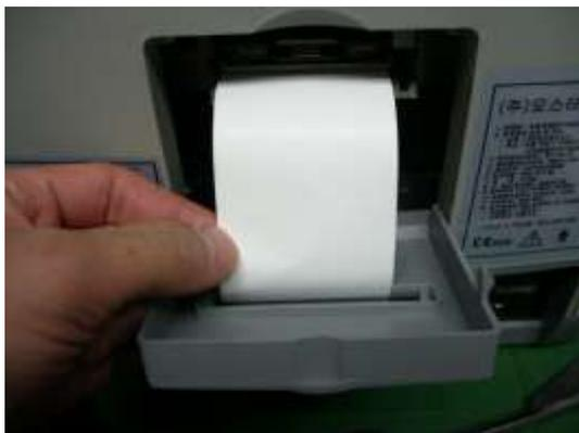
⑥ Paper cutting : For a sharp outline of report printing, cut off the remained paper once by a saw tooth in the cover.
