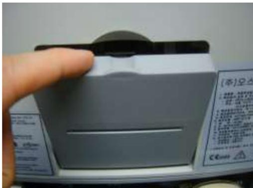
② Paper inserting : Insert the paper as shown below.
