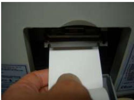
③ Cover shutting : Put the paper to the gap in the cover, then shut the cover up.
