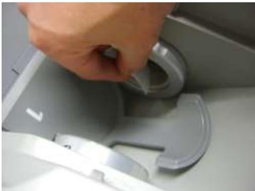
Clean the surface of the Coupling Pad with an alcohol pad and apply sufficient gel to probes.
