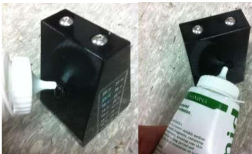
**Put the phantom on the foot supporter 1 (don't use foot supporter 2 when dailytest) in the measuring position of device.**
