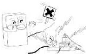
**For escaping from electronic noise, do not install near a electronic generator, X-ray equipment, broadcasting equipment. It causes a result to be inaccurate.**
