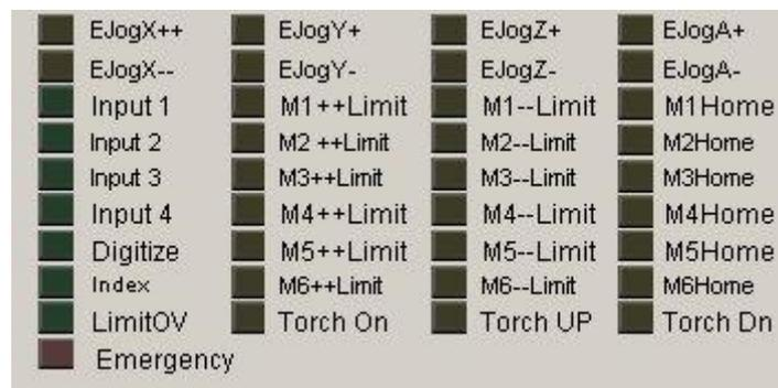
If the GND line contact with sensor, confirm the "Digitize" turns on. It is normal.
