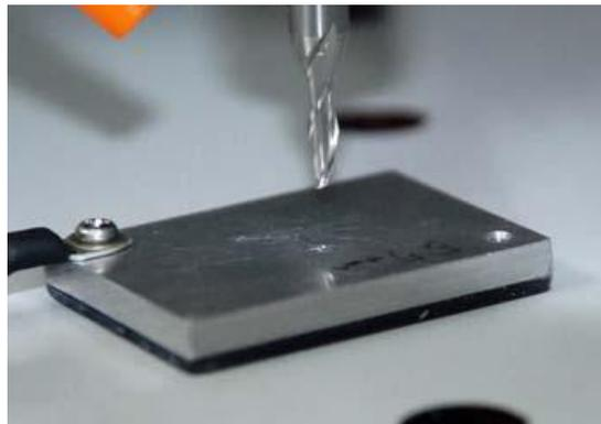
Set “Probe” to Input Signal in the Config→Port & Pins
