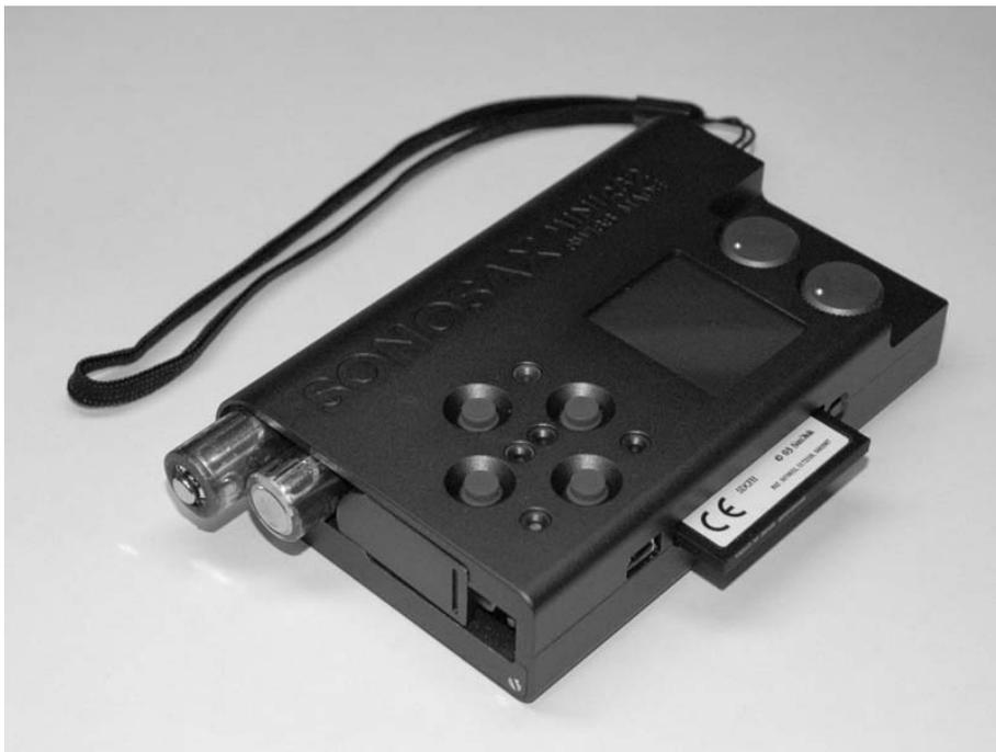
*External DC supply :* The MINIR82 can also be supplied from an external suitable DC source from 5 to 9 V. A 2 meter long cable with the DC plug is available, part nr V980010. For use with high capacity 12V battery, a 9V to 18V DC/DC converter will soon be available.
